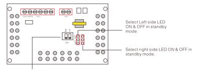
Jumper 1: alarm tone select(1 tone or 6 tone); Jumper 2: Cut off power alarm ON or OFF
