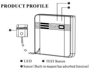
Sensor (Burit-in magnet has ausorbed function
