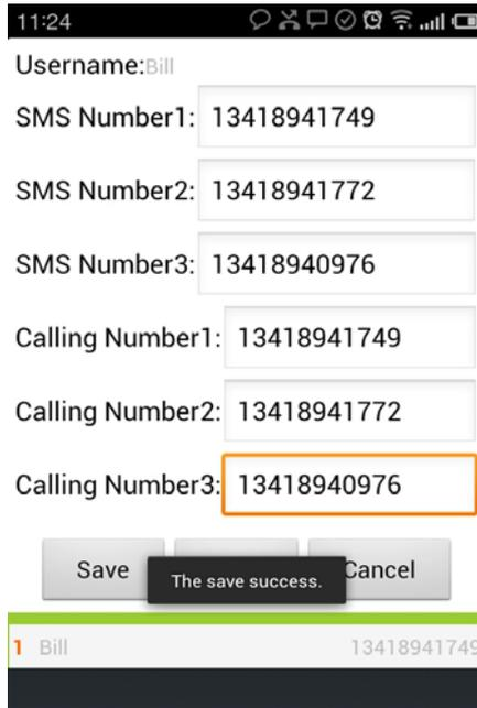
After finishing input, click “send”. After setting successfully, the alarm host will send out a confirmation message to the first message alarm cell phone number. Such as above image, the alarm host will send a setting information to the cell phone number 13418941749.
